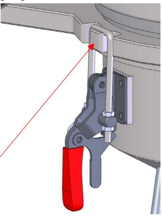
Easy fixation of WIP-drain with quick clamps
