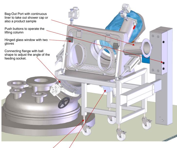
Height adjustable wheels to connect the system at the feeding socket
